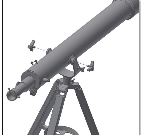
Figure 5. Secure the tube with the supplied hand knobs.
