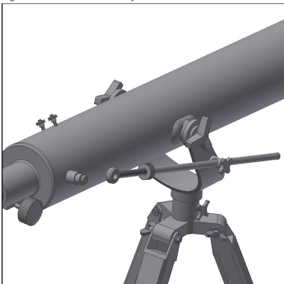
Figure 6. Insert fine focusing shaft.
