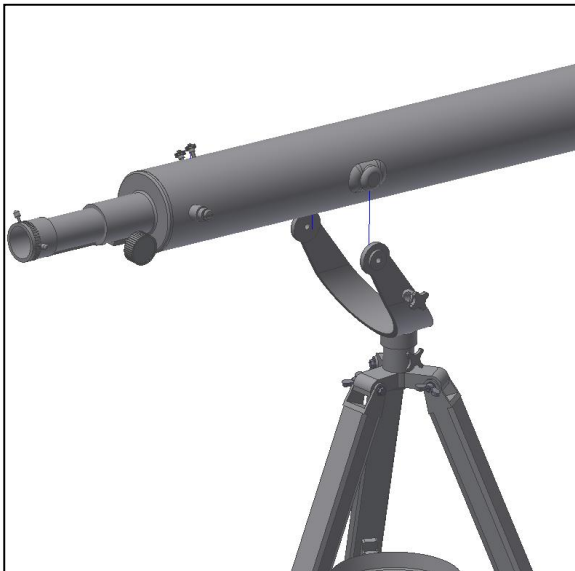
Figure 4. Place tube on the fork mount.
